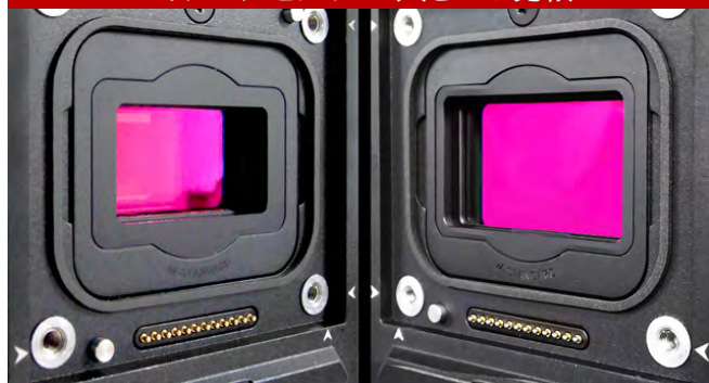
左: HELIUM 8K S35 (29.90x15.77mm/対角線: 33.8mm) 右: MONSTRO 8K VV (40.96x21.60mm/対角線: 46.31mm)
